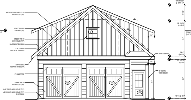
1 PROPOSED FRONT ELEVATION (HOUSE FACING) 1/4" = 1'-0"
