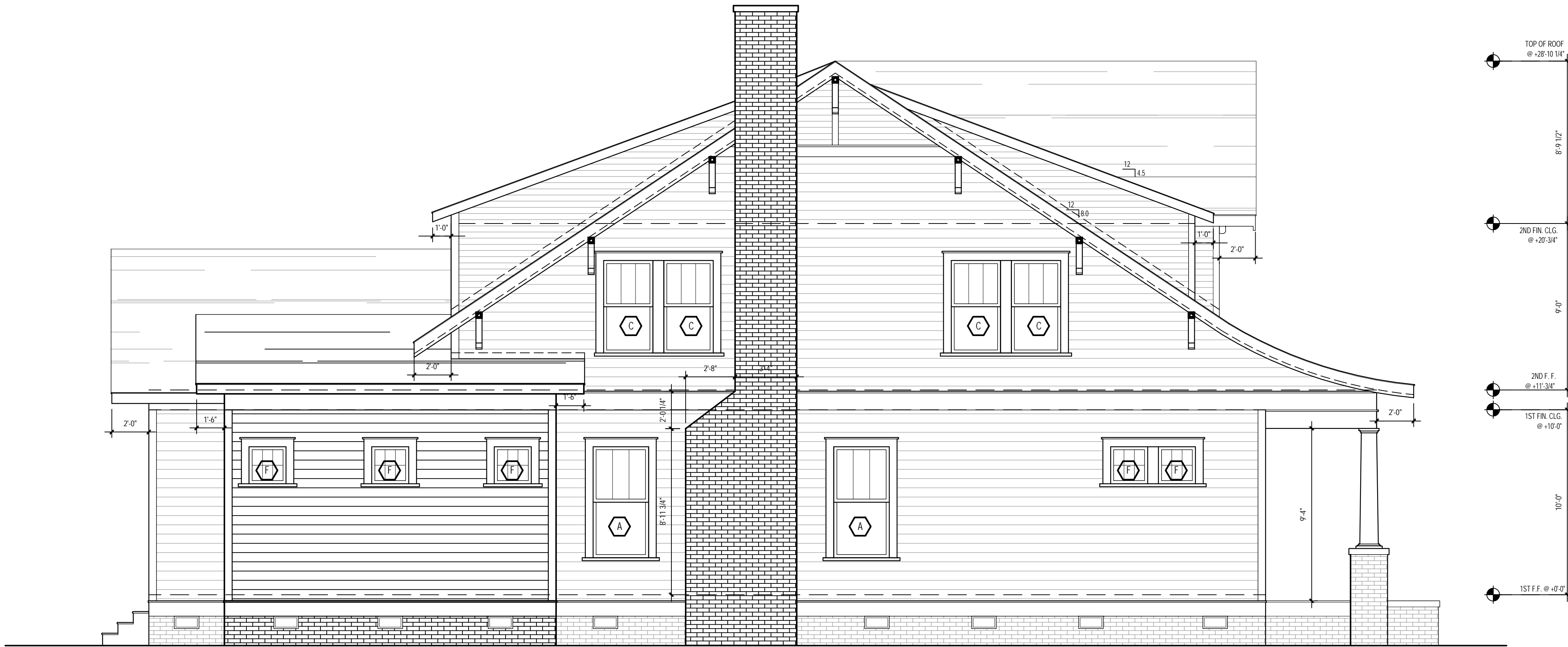
2 PROPOSED LEFT ELEVATION 1/4" = 1'-0"
