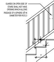
2 WOOD STAIR DETAIL (Interior) 3/4" = 1'-0"
